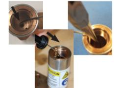
**17** Ensure that the Weld Pin moves freely up and down inside the Weld Body (with no constraint from the LVDT Cable Assembly). Then, thread on the Electrode Head and tighten to the corresponding torque (according to the weld body series):
