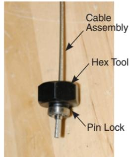
**13** Using a wrench to turn the Hex Tool, thread the Pin Lock (with the Cable Assembly) onto the base of the Weld Pin, being careful not to cross the threads. Wipe off any excess Loctite.
